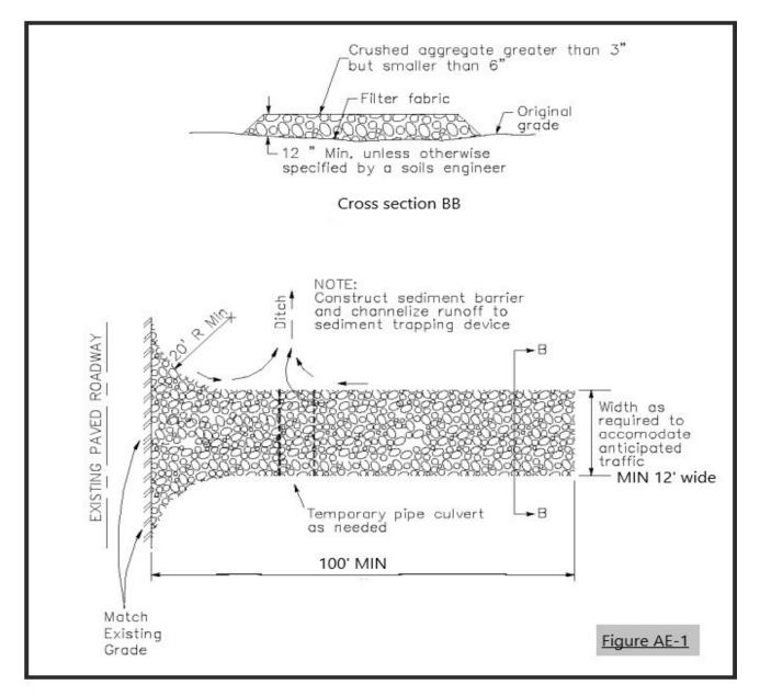
Inspections shall be made daily to ensure that mud and dirt are not tracked into the public roadway; top dressing may be required especially if the subgrade is soft or becomes saturated; daily cleaning of the public roadway of any residual mud and dirt. Do not wash excess mud and dirt into the storm water road drainage swales or nearby streams and rivers.
